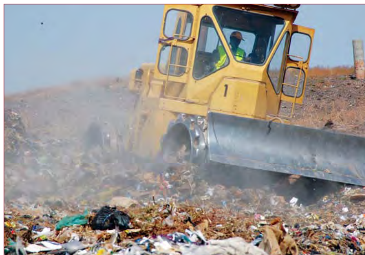
Daily operation of a landfill requires heavy machinery to place and compact the incoming waste
